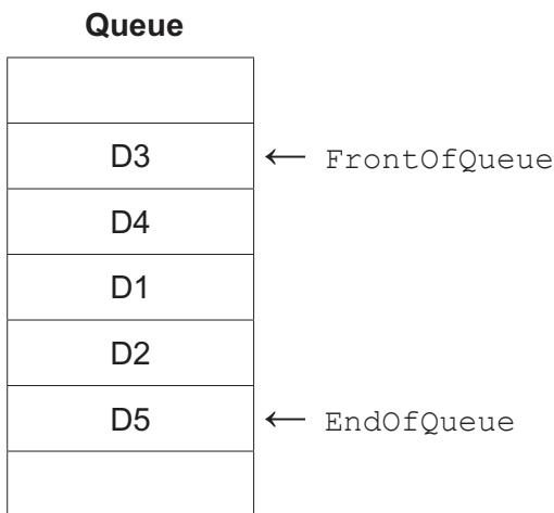
The queue is implemented using three variables and a 1D array of eight elements as shown. The variable `NumItems` stores the number of items in the queue.
